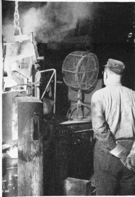
Bill Linskey, operator, stands by as the ladle with nearly a ton of liquid brass — ten times as hot as boiling water — is tipped, spilling its contents into the furnace. The ladle is tipped, as shown, by hydraulic mechanism.
